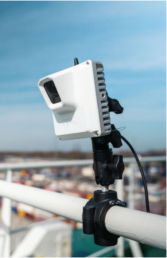
ADIS (Automated Debris Imaging System) camera
