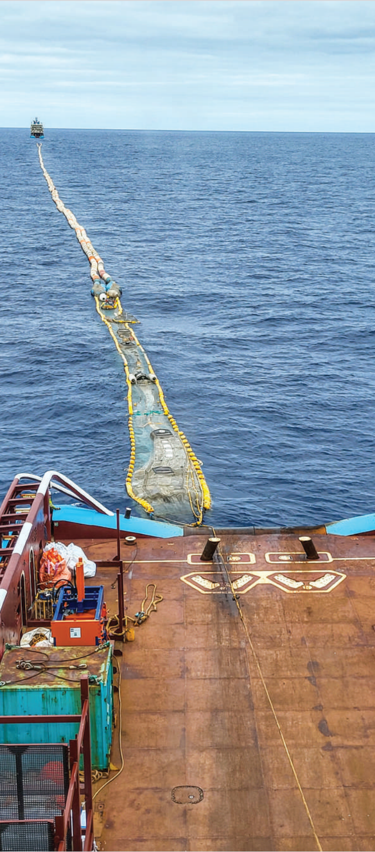
System 03 Retention Zone, filled with plastic and ready to be pulled on deck
