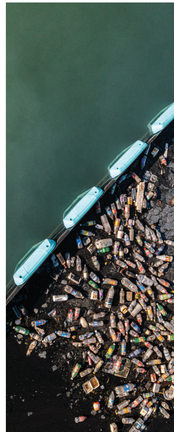
Top view of Interceptor 010. A barrier installed in Barnes Gully, Kingston, Jamaica
