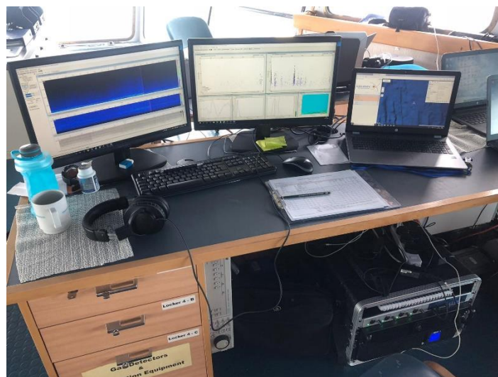
Figure 5 - Acoustic monitoring station on the bridge of Maersk Transporter
