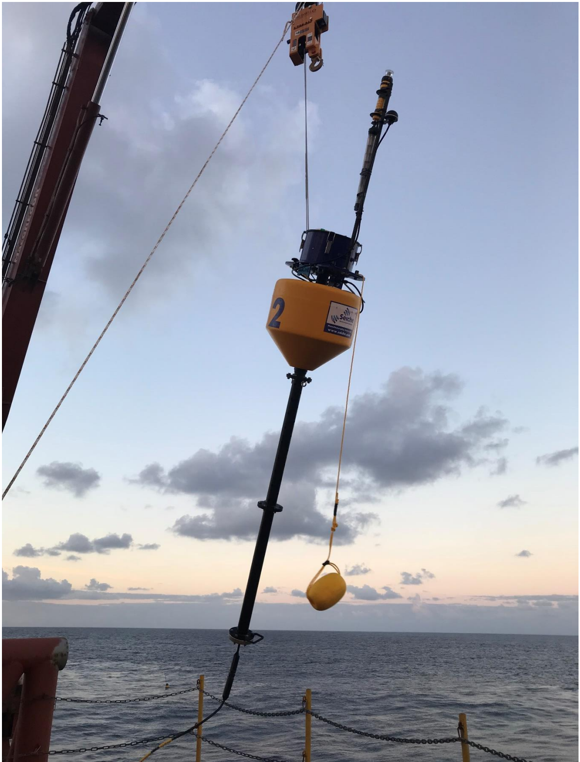
Figure 10 - PAM buoy recovery from Maersk Launcher
