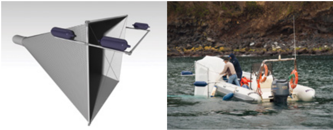
Figure 7.3 Trawl: a) Computer rendering of the trawl design, showing the metal frame, to which a net and fenders have been attached, b) deployment of trawl.
