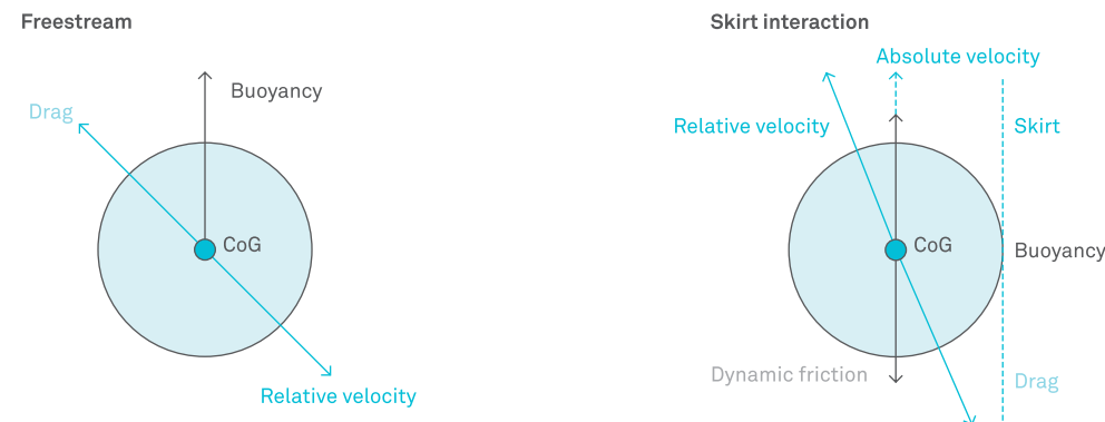
Figure 3.12 Sketch of forces on particle in free stream (left) and with wall interaction considering equilibrium of stream-wise forces (force of the fluid on the particle + barrier reaction) (right). CoG = center of gravity.
