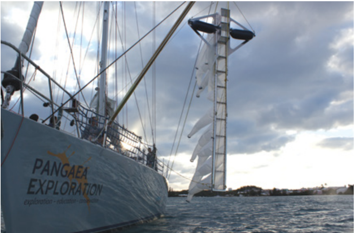
Figure 2.11 Multi-level Trawl attached to the spinnaker pole of vessel Sea Dragon, for the first expedition through the North Atlantic Gyre. Please note that the boxes in front of the top two nets were removed after testing, and hence were not used during trawling. Please note the extension boxes on net 1 and 2 pictured here were removed during sampling. Photo by Allard Faas.
