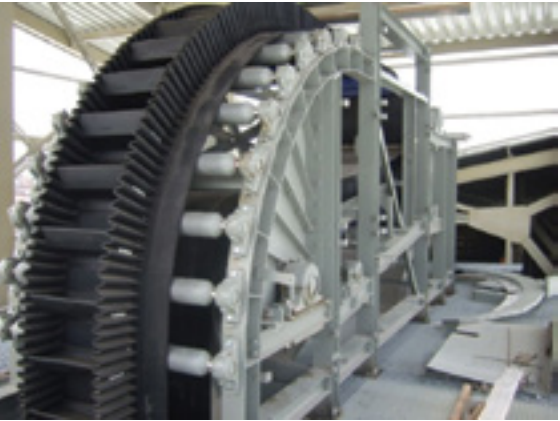
Figure 4.4 Pocket belt conveyor. Courtesy of Loibl Allen-Sherman-Hoff GmbH.
