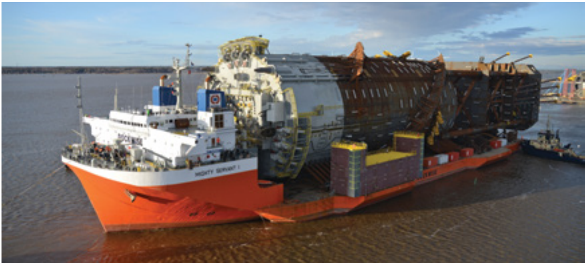
Figure 5.4 Spar transport using a heavy transport vessel
