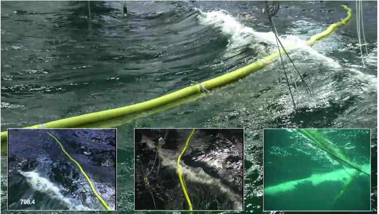
Figure 7-1: High mooring low pretension 225 deg ULS
