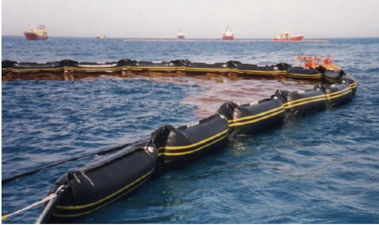
Figure 2. An oil containment boom (RO-BOOM 3500) in use. A similar boom will be used for the Prototype North Sea (picture from Ro-Clean Desmi 2001).
